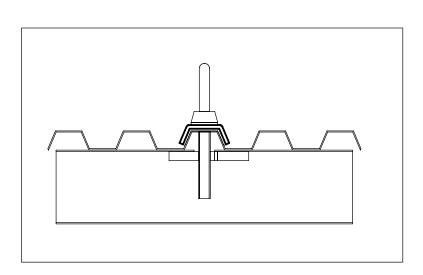
Spandeck type of Roof Deck with Folded type of flange. Hole to be drilled through crest of Roof Deck.
