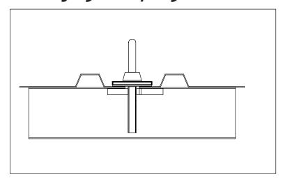
Standard Tray Deck Roof with Standard Round flange. Hole to drilled into centre of pan.
